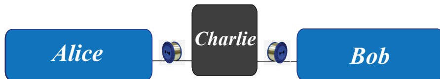
Figure 4.1.1. Schematics for MDI-QKD. Charlie facilitates the key distribution between Alice and Bob without being able to learn the secret key.
