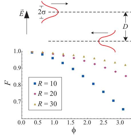
FIG. 3. (Color online) Introducing a transverse separation between the two pulses greatly relaxes the trade-off between  $F$  and  $\phi$ , such that a phase of order  $\pi$  becomes compatible with high  $F$ . The dimensionless separation  $R$  is defined as  $\frac{D}{\sigma}$ . The interaction strength has to be increased significantly in order to compensate for the transverse separation.
