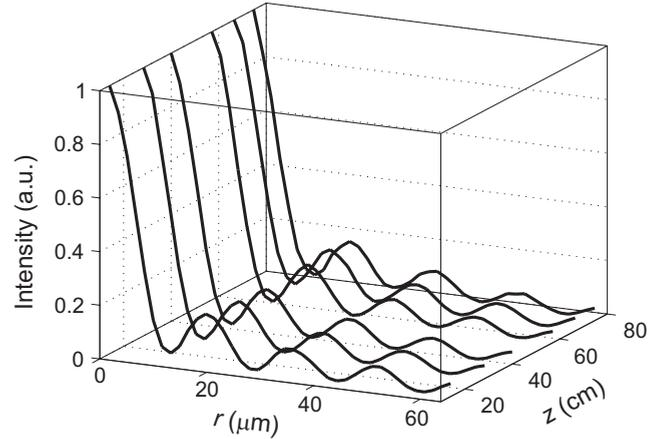
FIG. 2. Normalized radial intensity profile for several CCD camera positions.
