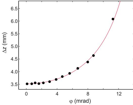
FIG. 4. (Color online) Cw measurements: period of the interference fringes  $\Delta z$  as a function of the angle  $\phi$  between the direction of propagation of the Gaussian and Bessel beams (dots) together with the theoretical fit (line).
