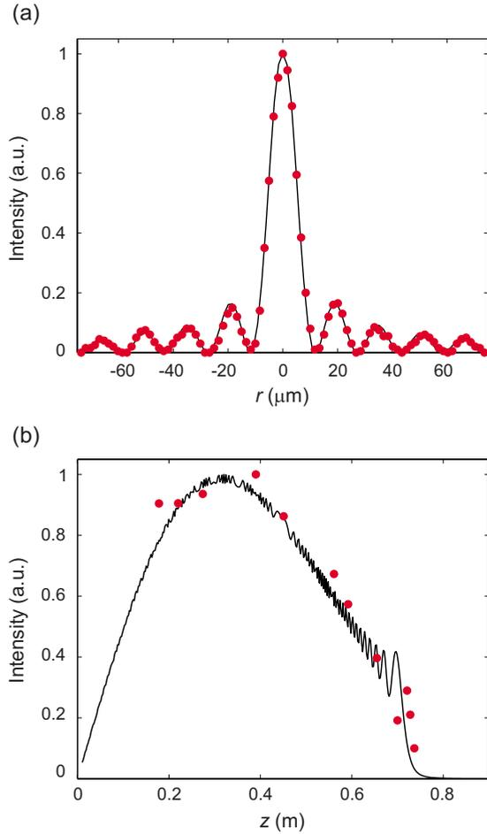
FIG. 3. (Color online) (a) Measured intensity profile (dots) and numerical calculation (line) at 18.8 cm distance from the conical mirror. (b) On-axis intensity: experimental data (dots) and theoretical calculation (line).
