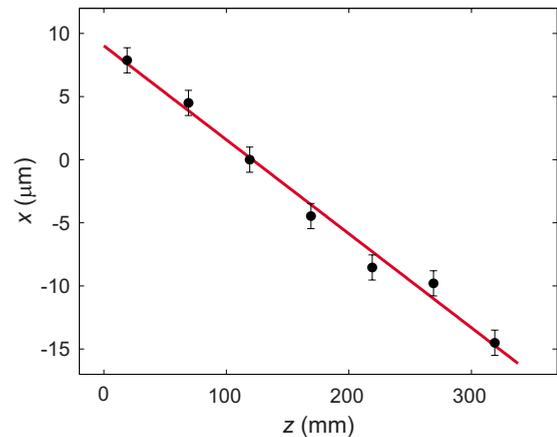
FIG. 6. (Color online) Displacement  $x$  of the Michelson interferometer plane mirror, at which the visibility is maximized, as a function of the CCD camera position  $z$  (dots) with a linear fit (line).
