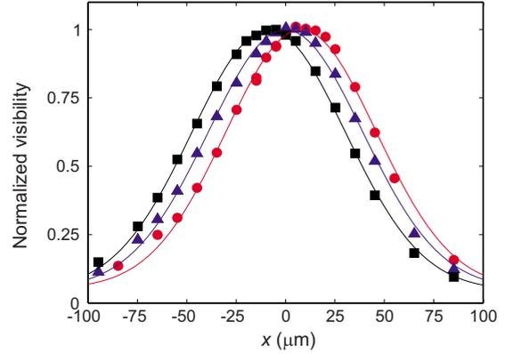
FIG. 5. (Color online) Pulsed measurements: normalized fringe visibility for  $z = 219$  (■),  $119$  (▲), and  $19$  (●) mm as a function of the plane mirror translation  $\Delta x$ . The experimental data are fitted with a Gaussian curve.
