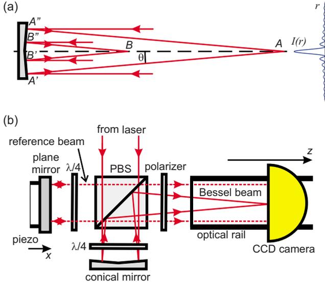
FIG. 1. (Color online) (a) Formation of the Bessel beam from a plane wave by a conical mirror and a plot of its radial intensity profile. (b) Schematic of experimental apparatus used for phase- and group-velocity measurements. PBS means polarizing beam splitter.
