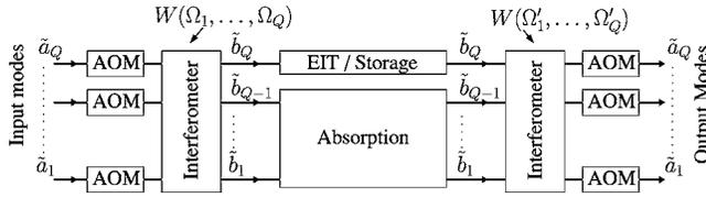
FIG. 4. Linear optical circuit equivalent to a multi- $\Lambda$  configuration. The phase shifts and reflectivities of the input (output) combining mirrors are determined by the phases and amplitudes of the classical control fields during the in-coupling (out-coupling) process. In this model, the acousto-optical modulators (AOM) at cell entrances and exits bring the input fields to the same frequency so they become indistinguishable when handled by the interferometers.
