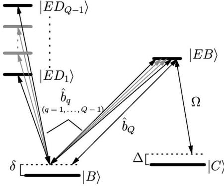
FIG. 3. The multi  $\Lambda$ -system after basis transformation of both atomic and optical Hilbert spaces: The classical fields  $\Omega_q$  drive only the  $|EB\rangle \leftrightarrow |C\rangle$  transition and form an EIT system with the quantized field mode  $\hat{b}_Q$ . The other modes  $\hat{b}_{q \neq Q}$  couple also to the excited dark states  $|ED_q\rangle$  and therefore undergo absorption.
