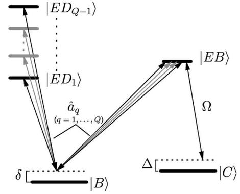
FIG. 2. Multi  $\Lambda$ -system in the excited dark-state basis: The classical fields  $\Omega_q$  drive only the  $|EB\rangle \leftrightarrow |C\rangle$  transition and each quantized field mode  $\hat{a}_q$  mode couples to all of the excited states  $|ED_{(1,\dots,Q-1)}\rangle$  and  $|EB\rangle$ .
