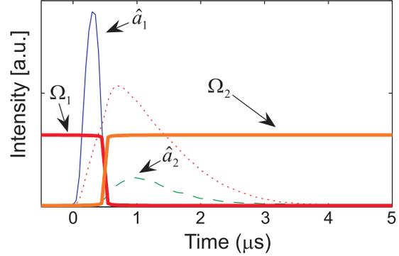
Figure 2: Implementation of RATOS. The two control pulses  $\Omega_1$  and  $\Omega_2$  are switched, respectively, off and on when the signal pulse  $\hat{a}_1$  (scaled down) is inside the cell. Without switching the control fields, the signal pulse is slowed down (and partly absorbed) in the Rb cell, giving rise to the pulse shown by a dotted line. The created RATOS pulse is shown by the dashed line.
