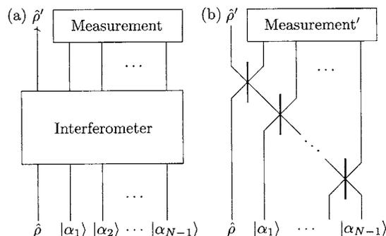
Fig. 2. (a) General setup for transforming the state  $\hat{\rho}$  to  $\hat{\rho}'$ , involving an interferometer and a conditional measurement. (b) Same interferometer after absorbing all but a line of beam splitters into the measurement.
