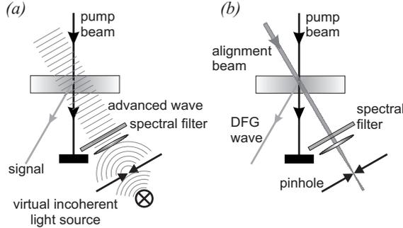
**Figure 2.** (a) Interaction of Klyshko's advanced wave with the pump generates a DFG mode that mimics that of the CPP. (b) In an experiment, the role of the advanced wave can be played by a laser beam, aligned so as to obtain maximum transmission through all the filters.
