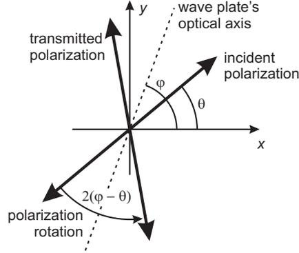
Figure A.2: Polarization rotation by a  $\lambda/2$  plate.**Quarter-wave plate**
