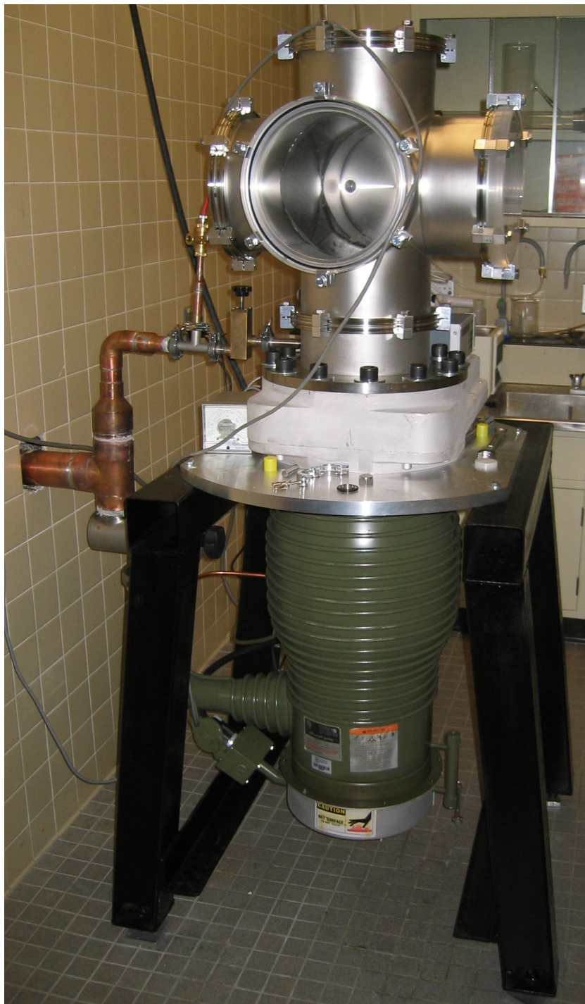
Figure 3.5: Photograph of the vacuum system showing the six-way vacuum chamber, diffusion pump, and the pneumatic gate valve in the middle.
